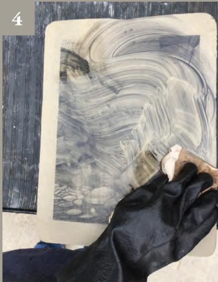
3. The printer coats the surface of the stone and drawing with gum arabic and nitric acid, a process that treats the non-drawn areas of the stone so that it will attract water and repel ink.
